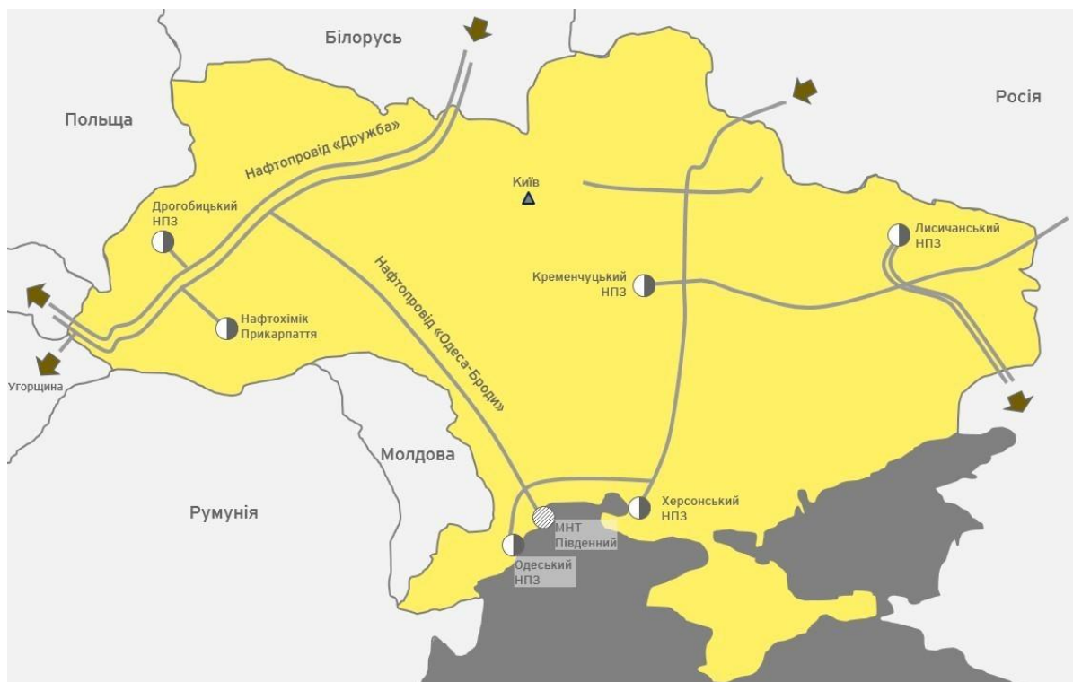
Figure 5-23: Scheme of the main Ukrainian trunk pipelines 100
